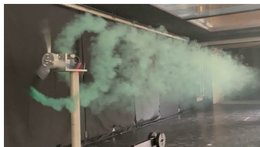
Fig. 1. Wind turbine wake by wind tunnel experiment.
